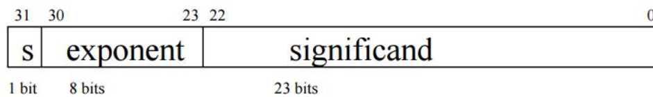
Figure 8.2: Source: The template for representing a number in scientific notation using the IEEE 754 standard for a 32-bit string. Courtesy of Prof. Mann's slides.
